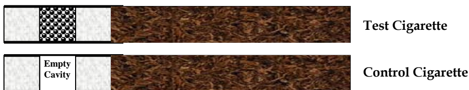
Figure 1: Schematic representation of the test cigarette incorporating a granular additive and the control cigarette consisting of an empty cavity
